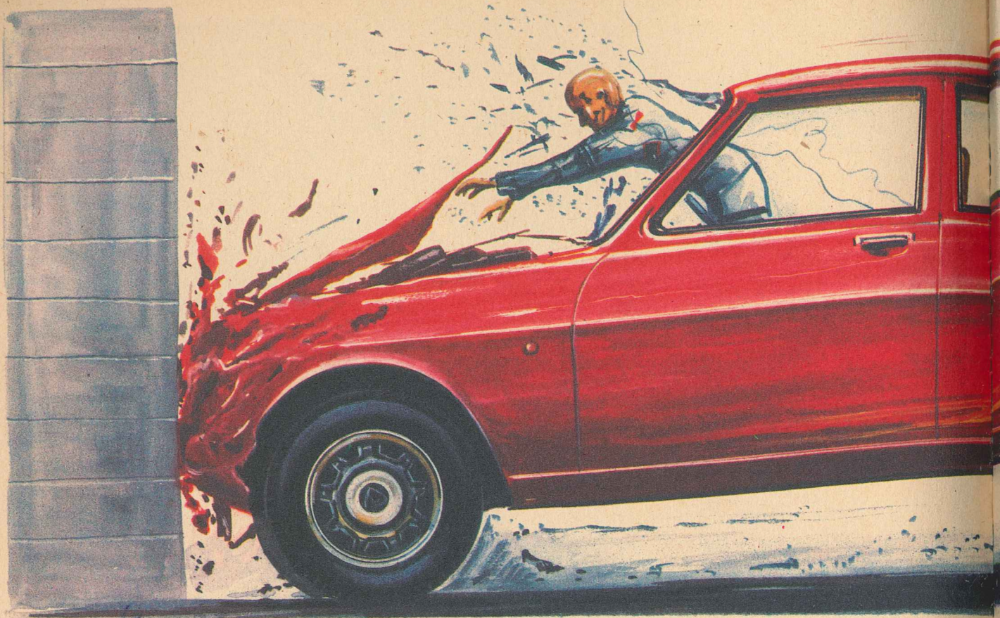
A car being tested for safety by staging a mock crash and using a dummy in the place of the driver. A typical car-testing dummy, showing the photographic markings on the head, face and other injury areas.
